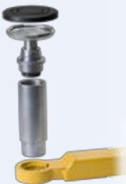
CL10V3-DPC models come standard with double telescoping screw with removable pad and 10315 Stack Adapter Kit - includes (4) 3" adapters, (2) 6" adapters and (2) organizer racks.
