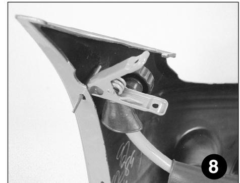
**Clamps and/or Pins.** Use pins to secure bumpers when possible to assure full paint coverage. Maximum weight 25 pounds.
