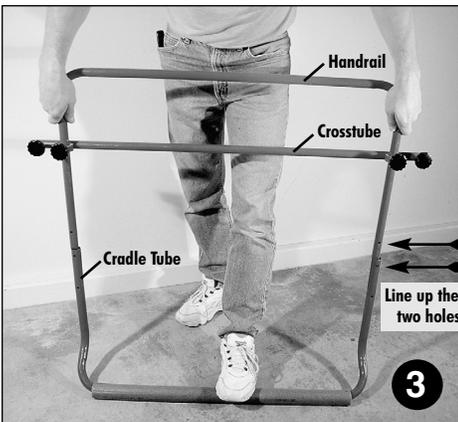
**Cradle Assembly.** Slide handrail into crosstube. Insert two plastic knobs, then tighten. Then slide handrail into cradle tube only to first hole (see arrows in photo).
