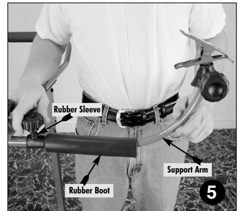
**Install Support Arms.** Rubber boots (P/N 220-029) onto crosstube. Slide support arms into crosstube. Insert rubber sleeves and tighten plastic knobs.
