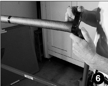
**Mounting Foam Pad.** Electrical tape can be used to better secure the foam pad to the upper cradle tube.
