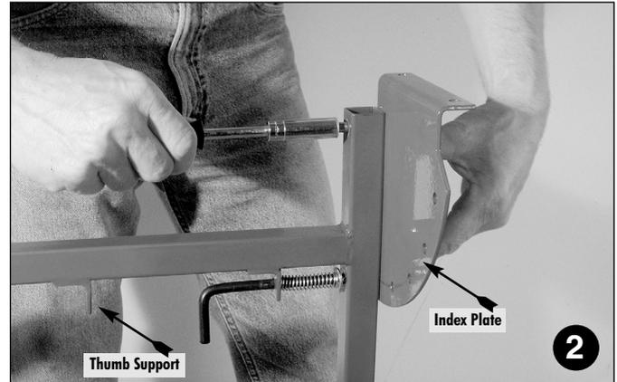
**Install Index Plate.** Use a  $\frac{7}{16}$  socket to slide push clip onto the index plate rivet.
