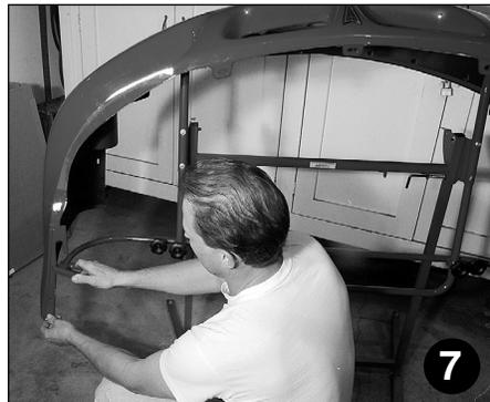
**Mounting Bumper Cover.** With the cradle support in a downward position, center the bumper cover on the foam pad. Adjust crosstube to proper length of bumper ends. Tighten knobs. Adjust support arms to proper width of bumper and tighten knobs.
