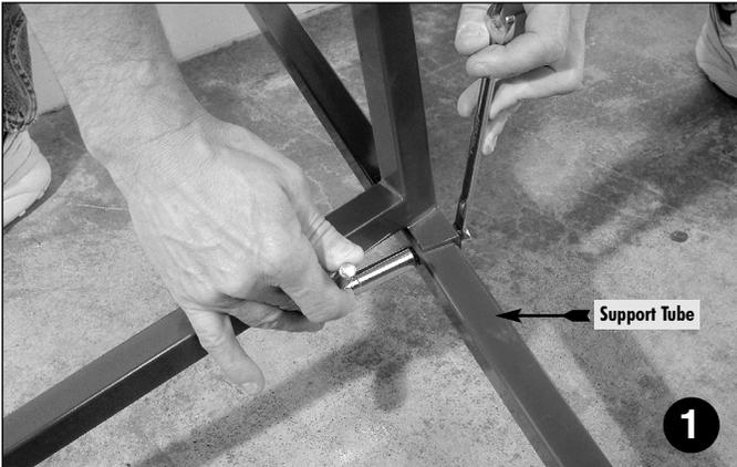
**Install Support Tubes.** Install plastic end caps and bolt on the foot pads using  $\frac{1}{4}$ " flat washer with nut. Then, using four  $1\frac{1}{2}$ " bolts with washer and nuts, mount support tube to frame. Then, install wheels.
