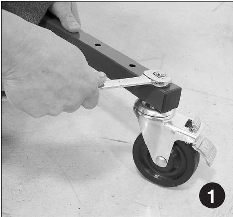
1 Install wheels to leg support tubes.
