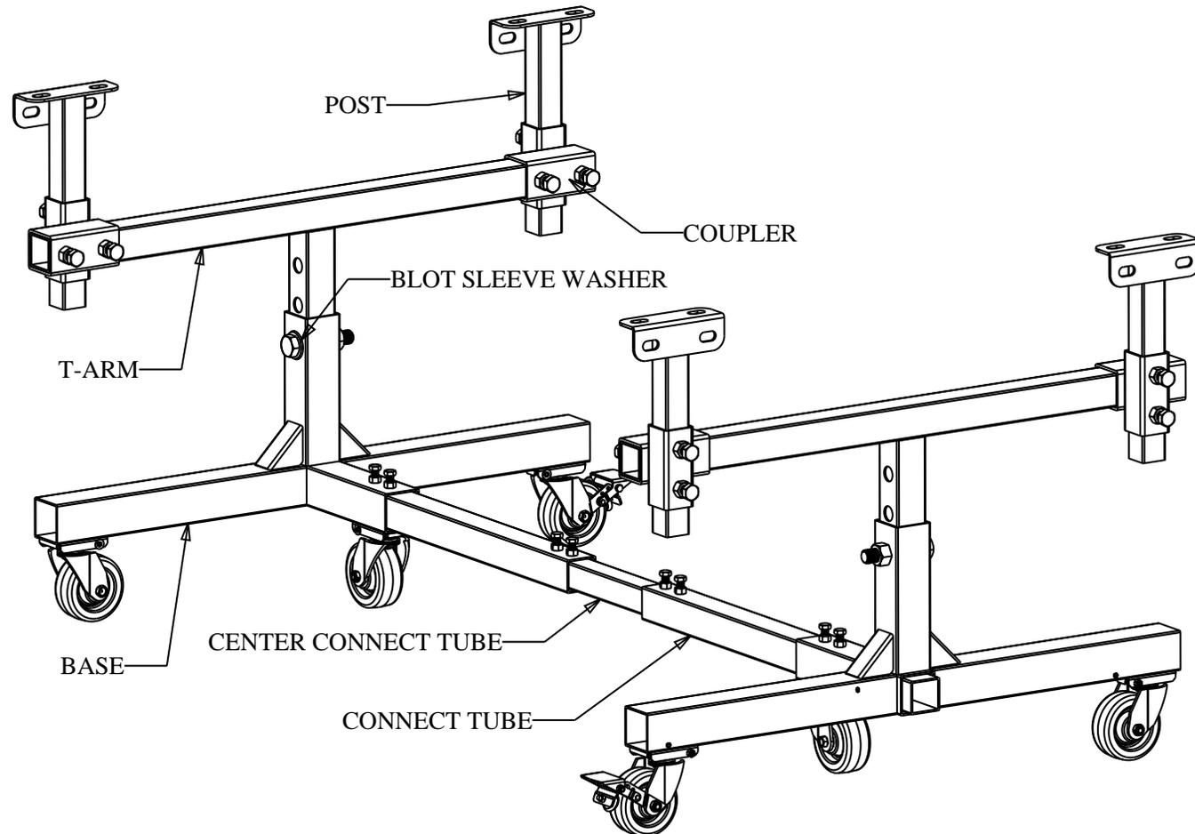
The Body Cart Plus comes packaged on a pallet. The Center Connect Tube & Connect Tubes are packed on top. The mounting arms are rotated down 90 degrees for shipping. The wheels & hardware are in the box, strapped to the pallet.
