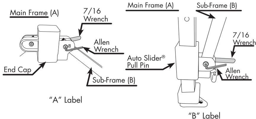
Attach the Main Frame (A) to the Sub-Frame (B) at each of the six connection points:
