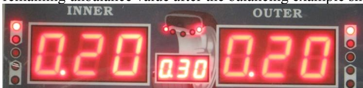
As you can see, the wheel is still technically out of balance by .20 Ounces on both sides. However, because I had the “least unbalance value setting” on .70 Ounces, the machine ignored the remaining .20 ounces because it was less than .70 ounces.
