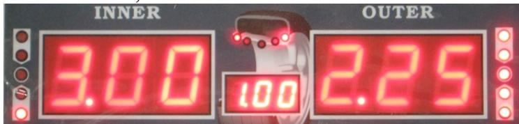
Then place the 2.25 Ounce weight that came with the machine at 12 o'clock on the outside of the rim using the provided wheel hammer. After placing the weight, close the hood and spin the wheel. The following screen will appear:
