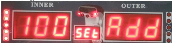
Then place the 100gram or 3.5 Ounce weight that came with the machine at 12 O'clock on the inside of the rim using the provided wheel hammer. 100 grams = 3.5 ounces so either weight is ok. Remember that at anytime you can switch from Grams to Ounces and back by just pushing the C button.
