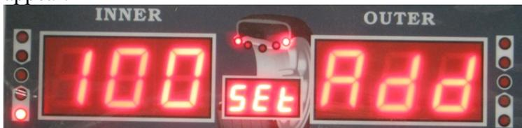
Remove the weight from the outside of the rim. Use your hand to rotate the tire until all 5 of the lights in the **INSIDE UNBALANCE POINT** are on, as shown here:
