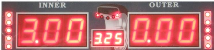
Now place the 3.00 Ounce weight that came with the machine at 12 o'clock on the outside of the rim using the provided wheel hammer. After placing the weight, close the hood and spin the wheel. The following screen will appear:
