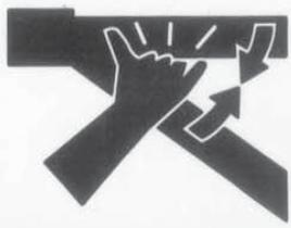
Keep clear of pinch points when lift is moving.
