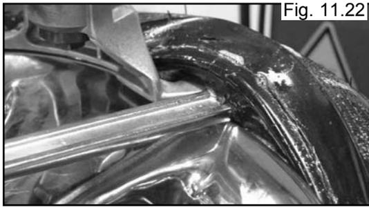
21. Depress the table top pedal to rotate the wheel clockwise. Leave the right hand helper in position opposite the demount head and allow it to follow the wheel rotation to assist the bead into drop center while demounting. Hold the tool bar down until demounting nears completion. (See Fig.11.23 - 11.25)
