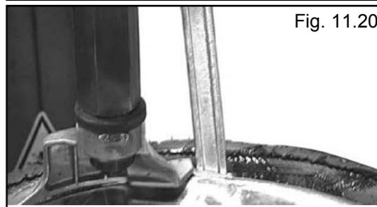
20. Push the tool bar down toward the wheel to lift the tire bead up and over the right -side knob portion of the demount head. Hold the tool bar in this position. (See Fig. 11.21 - 11.22)
