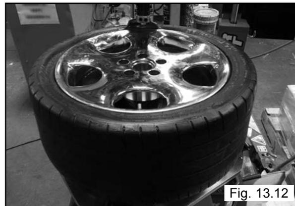
8. Depress the table top pedal and rotate the tire until the bead is mounted. The right side helper shoe will follow the tire during rotation. (See Fig. 13.9 -13.12)
