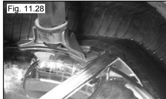
24. Depress the table top pedal to rotate the wheel. The demount head will guide the bead up and over the edge of the wheel. Continue rotation until the lower bead is de-mounted. The helper disk should be removed during rotation. Swing the disc out of the way to complete de-mounting. (See Fig. 11.29)
