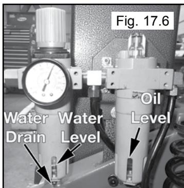
3. Add oil to the lubricator if the fluid level is below the middle of the sight glass. Remove the reservoir by turning counter-clockwise and pulling down. Add SAE 10W non-detergent oil or an air tool oil if necessary.
