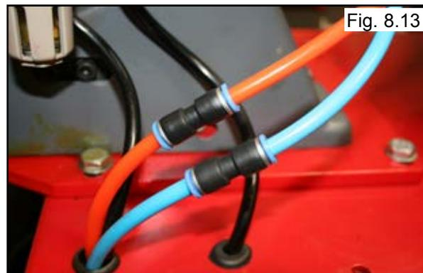
16. Connect the Air Line from the Tilt Back Tower to the Tee Fitting located Inside the Rear of the Cabinet. (See Fig 8.15)
