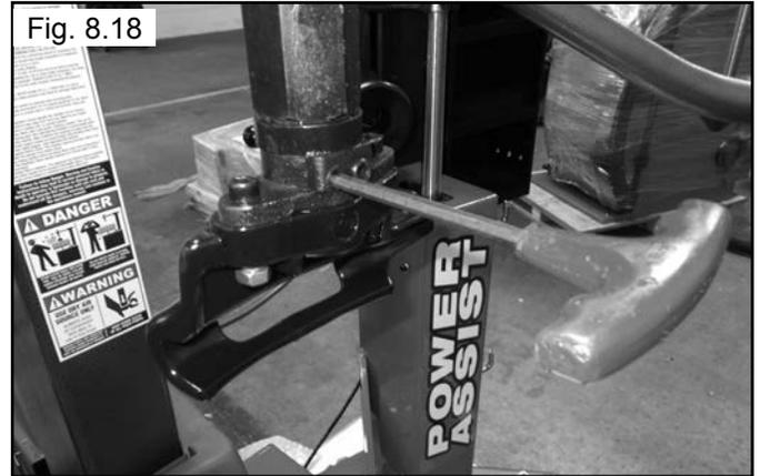
4. Once the plastic demount head has been removed you can place the metal demount head in place. Make sure the top of the demount head is pressed firmly against the plastic hex shaft spacer and tighten both the allen set screws and the bottom hex nut. (See Fig. 8.19)
