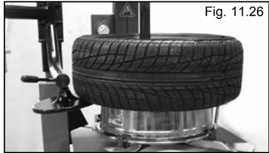
23. Insert the smooth curved end of the tool bar over the right end of demount head and below the lower bead of the tire. Push the tool bar down toward the wheel to lift the tire bead up and over the right-side knob portion of the demount head. Hold the tool bar in this position. (See Fig. 11.27 -11.28)
