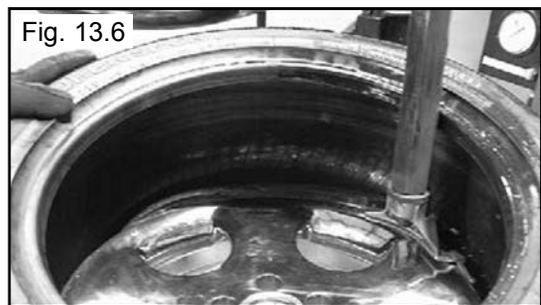
6. For the top bead, rotate the table top until the valve stem is directly across from the mount head. Lift the upper bead above the left "duckbill" side of the mount/demount head and below the right front knob. (See Fig. 13.7)
