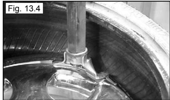
5. Manually force the tire down into the drop center of the wheel directly across from the mount head to reduce the tensional force on the bead. Depress the table top pedal and rotate the wheel to mount the lower bead. Rotate the table top until the lower bead is fully mounted. (See Fig. 13.5 -13.6 )
