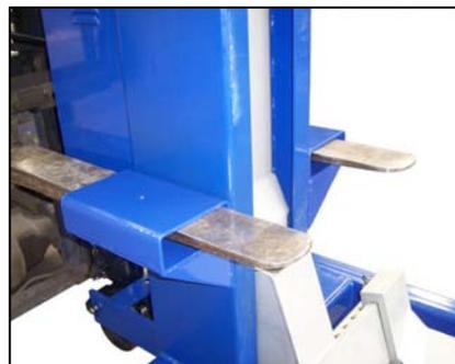
**Fig. 4a & 4b Forklift pockets on Column**
