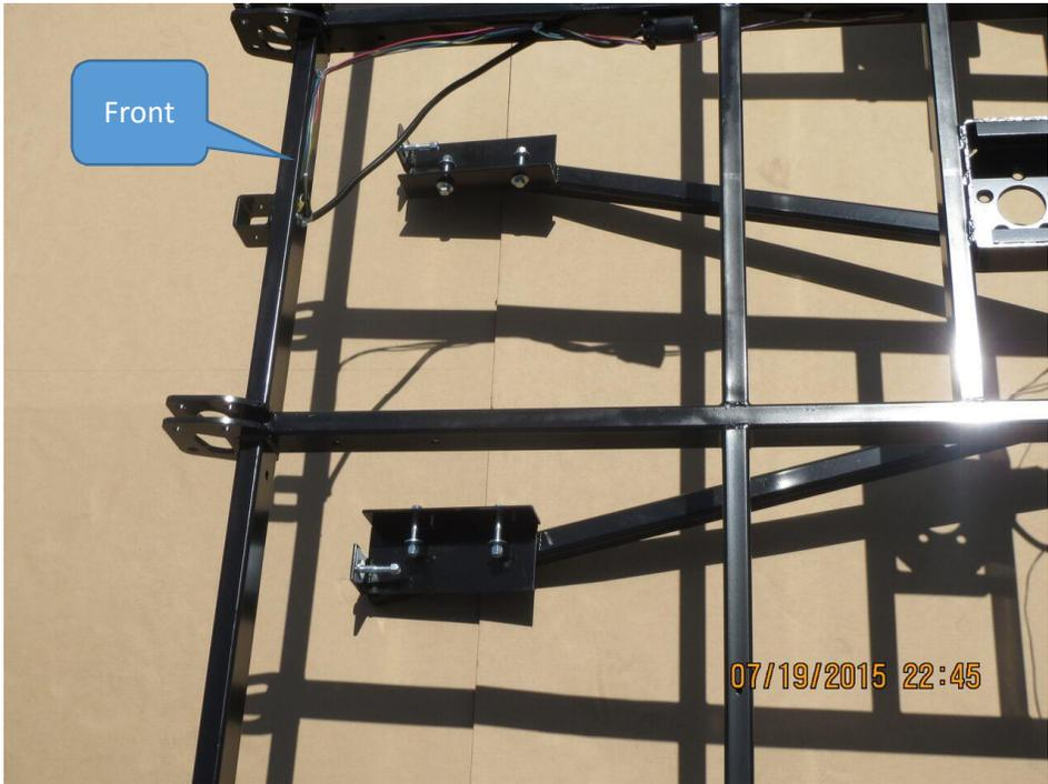
Lift the Tandem Tow frame up to the SWIVELWHEEL-58DW frame and clamp or block into position. With the supplied mounting bolts, bolt the system into place as shown in the following photos below. Once all mounting bolts are in position, tighten all nuts fully.
