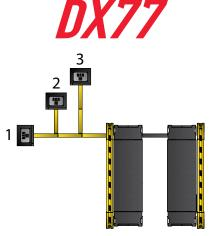
Manufacture provided 60" (standard length) air and hydraulic hoses allow three ergonomic, recommended power console placement options.
