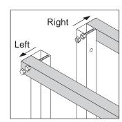
Horizontal posts are to be attached to the **outsides** of the vertical posts.
