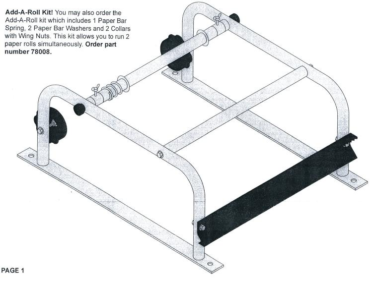
**STEP 1.** Assemble the main frame using 1/4"-20 X 2" bolts and 1/4" washers. **Note the locations of all punched holes** in all tubing to ensure proper assembly. Assemble and install the Tape Spools. Follow the diagram below closely to ensure proper assembly of the Tape Spools. The order of the hardware is identical for both sides.
