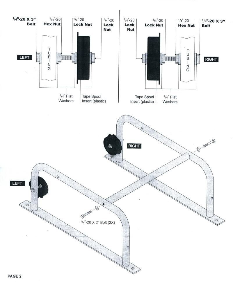
**STEP 2.** Assemble the rear Paper Bar following the diagram below. Attach rear Paper Bar to the Leg Assemblies using Knobs. Next, install Cutter Bar as illustrated below. Ensure that Cutter Bar teeth are on top and facing forward as shown. **You will install the Paper Bar Spring in the next step.**
