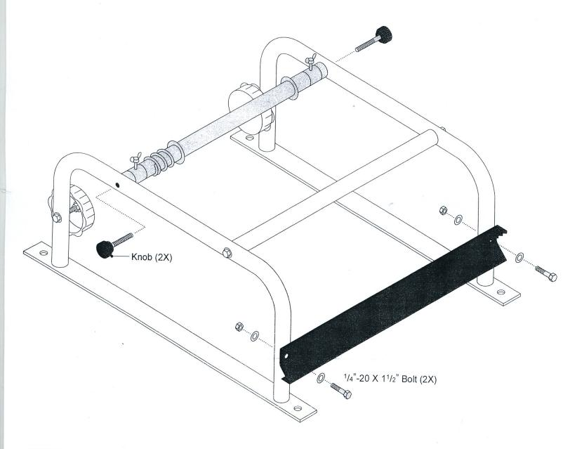
**Paper roll and Tape Spool placement.** Two Tape Spools are included so that you may conveniently run your tape along either end of your paper roll by simply adjusting the location of the paper roll along the Paper Bar.
