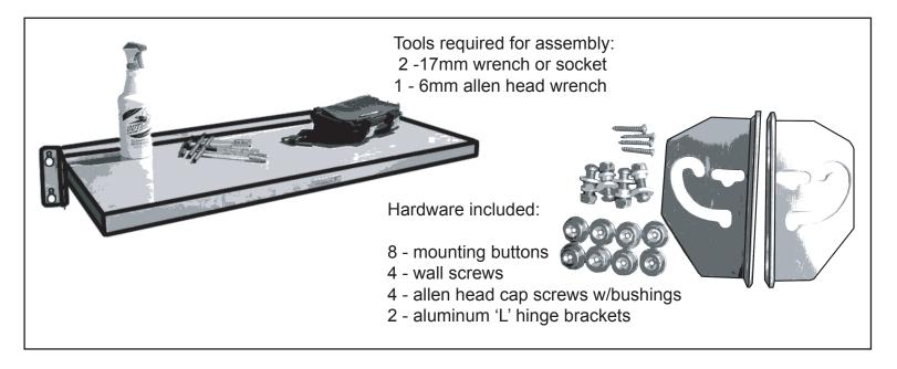
Mount 4 aluminum 'Mounting Buttons' to the wall using 48" centers between the 2 brackets. Each bracket should have buttons located 4.25" centers vertically. Table top will sit approximately at the level with the bottom portion of the upper 'keyhole' on the brackets so be sure to locate them at a comfortable working height. Extra 4 buttons are for 2nd mounting location to allow work bench to be easily moved and utilized.
