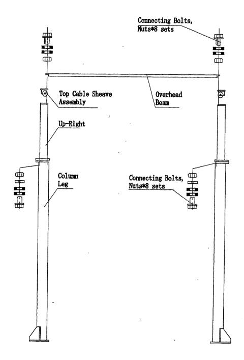
Equalizing Cable Installation - Overhead Beam Type
