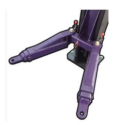
10. Ensure that arm restraint gear and arm gear have proper interlock and are functioning.
