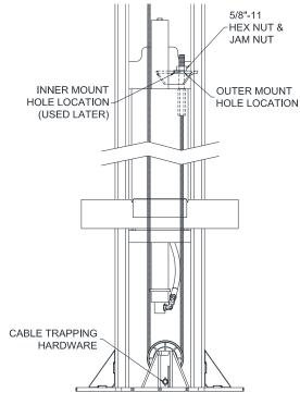
Fig. 2 – Cable Routing LAYOUT
