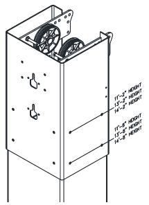
Fig. 3 – Column Extension Assembly
