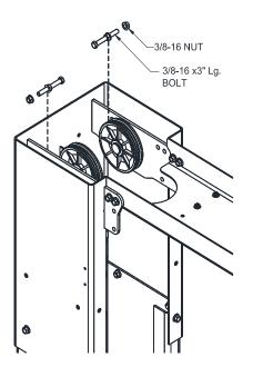
Fig. 8 – Column Ext. Cable Trapping
