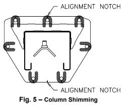
16) Tighten power column anchors and recheck column for plumb. Re-shim if necessary. Torque to 150 foot pounds to set anchors.
