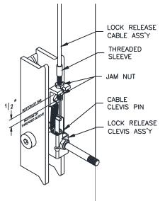
Fig. 13 – Power Column Lock Assembly
