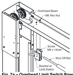
Fig. 7a – Overhead Limit Switch Power Side
