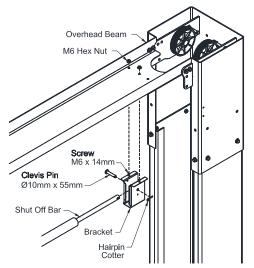
Fig. 7b – Overhead Bracket Idler Side
