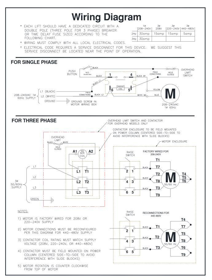
Fig. 16 – Electrical Wiring Diagram
