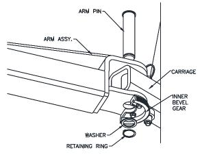
Fig. 15 – Arm Pin Keeper Install
