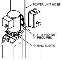
Fig. 10 – Power Unit Mounting
