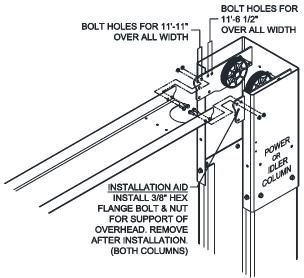
Fig 6 – Overhead Assembly
