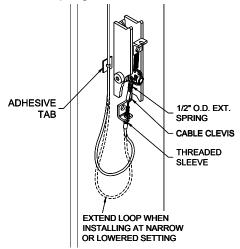
Fig. 14 – Idler Column Lock Assembly
