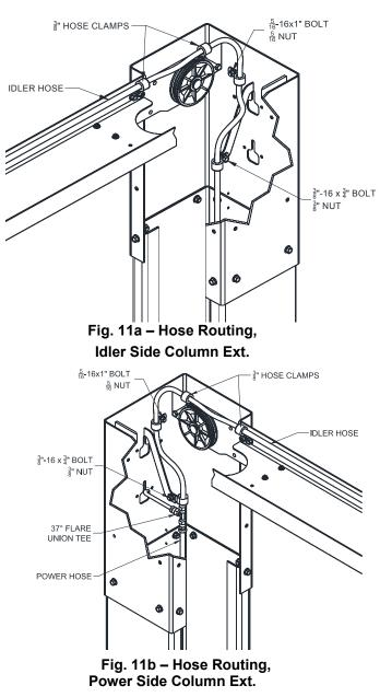
27) Loosely attach power column hose and idler column hose using the tee fitting (*in hardware box*) Attach Power Unit Hose to power side column extension as seen in Fig. 12. Connect Power unit hose to tee from Fig. 11b and remove slack from power column hose. Tighten loose fittings and clamps from previous step. Serpentine any extra hose length in overhead.
