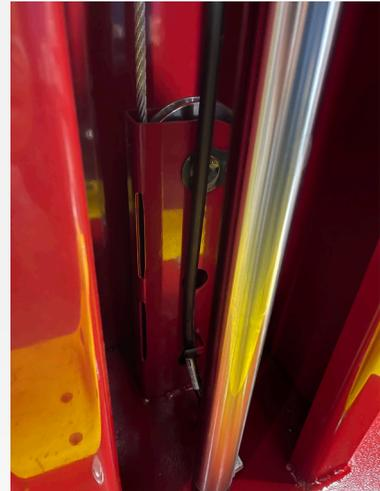
**Innovative synchronizer cable system** easily adjusts to any of the three lift height options without extra parts or making the cable connection inaccessible.
