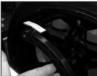
10. Pull the index arm out to the center plane position, the center **WIDTH** window will count down for you and display --0 when you have approached the correct position.
