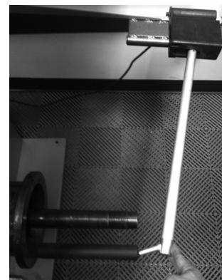
9. While holding the tip of the outer gauge arm onto the 200mm calibration attachment, press the **ALU** button.
