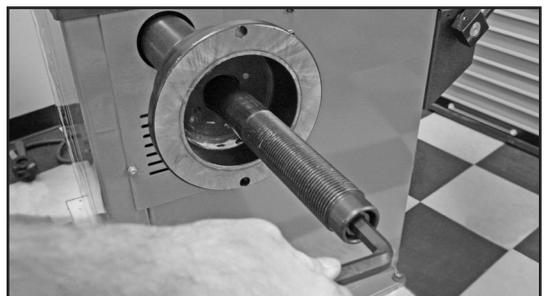
2. Locate and align the witness marks on the Face Plate and Shaft Assembly.
