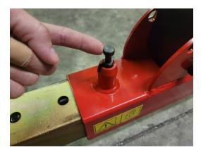
Should you choose to lower this pin into the locked position, it is imperative you do not forget you have done this and proceed to operate the machine by pumping on the hand pump. Doing so will surely cause damage to the machine by elongating the safety locking holes as shown below
