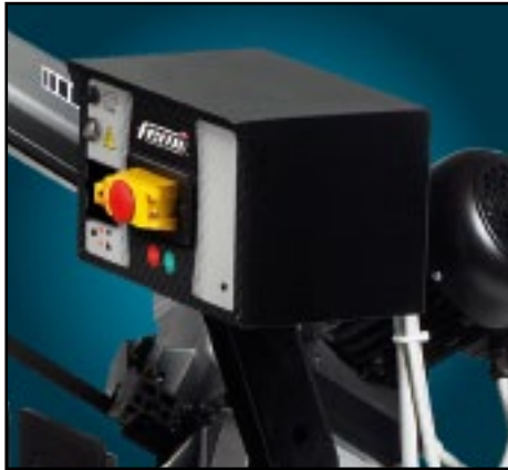
Single-phase induction motor with control panel.
