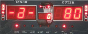
This parameter measures the distance of the wheel from the balancer. This is the A parameter. Use the built in ruler and extend it to the edge of the rim. You then multiply the measurement by 10 and enter than number for this parameter using the **UP** or **DOWN** key. For example if the ruler shows 8, you multiply this by 10 to get 80. Enter 80 as
