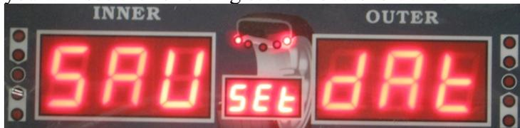
After showing this screen, the machine will automatically return to the initial balancing screen. You have successfully calibrated the machine and the data was saved automatically. The numbers you now see on the screen is the reading of unbalance of the
