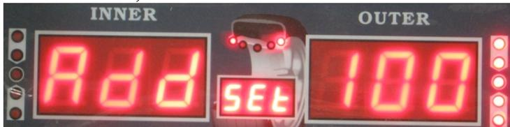
Then place the 100gram or 3.5 Ounce weight that came with the machine at 12 O'clock on the outside of the rim using the provided wheel hammer. 100 grams = 3.5 ounces so either weight is ok. Remember that at anytime you can switch from Grams to Ounces and back by just pushing the C button.
