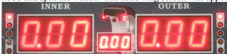
You zeroed out both sides and successfully balanced the wheel.
