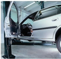
Asymmetric lifting allows easy access for interior work
