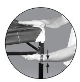
**7.** To engage the slider at each corner, first lift the fabric off of the corner, then with one hand hold the top of the leg while pushing up on the slider with the other hand. The pull pin will engage the hole. Pull down the fabric valance over the slider. Repeat on all four corners.
