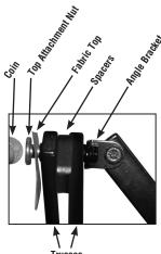
\*5. Unscrew top attachment nut from bolt. Place grommeted fabric top over the bolt, screw on top attachment nut and tighten until snug. Top should rotate easily - do not overtighten. Repeat this procedure on the remaining grommets.
