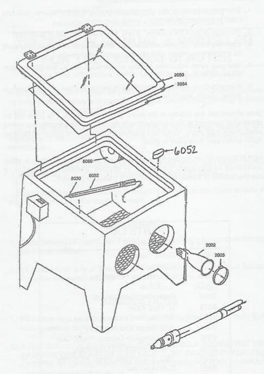
If media is slow to draw up the tube - begin covering the hole with the sleeve. If the media is clumping and the spray is surging - uncover the hole a bit.
