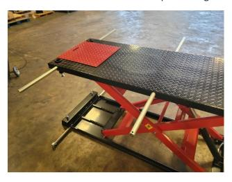
Again, using the supplied hardware you'll insert all 4 clevis and cotter pins, effectively pinning the side extensions into place so that they cannot possibly slide off without intentionally doing so.
