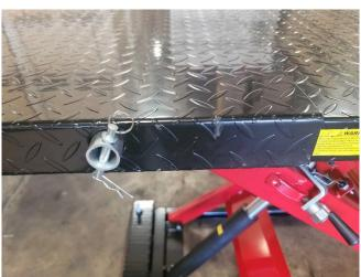
Next, you'll insert the middle length pole into the base of the machine. This is an anti-tip stabilizer bar.
