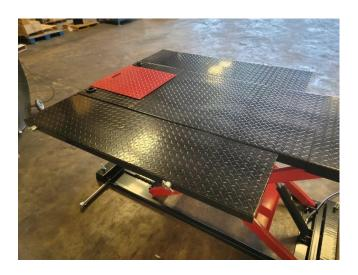
Next, you'll attach the 3 piece ramp assembly to the table top as shown using the hooks of the ramps to drop into the holes in the table top, as well as the holes in the side extensions
