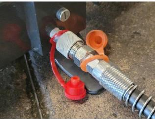
Next, be sure to pull the small brass-colored vent into the upward position as shown. This allows the pump reservoir to breathe and allows air to come in and out of the reservoir during operation.
