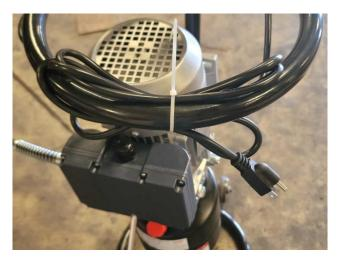
On the optional electric pump upgrade, the green button will raise the lift, and the red button kills power to the motor, and the lever with black ball knob at the end will lower the lift.
