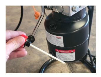
The electric pump already comes with a substantial amount of electrical cord. We do not recommend using a long, thin extension cord to operate the electric pump as you may experience significant "amp loss" and harm the motor. If you're going to use an extension cord, the shorter and thicker the size of the cord, the better.
