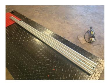
You'll insert the shortest pole through the front extension panel and also through the lift table at the same time, resulting in the shortest pole slightly exiting the front extension panel on both sides. Once done, you'll insert the provided clevis pin and cotter pin on each side of the front extension support pole
