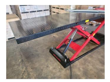
Be sure to line up the large holes on the sides of the front extension panel with the same holes found in the lift table.
