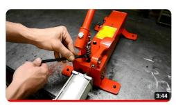
Priming the Redline 1500HD Pump & Raising the Release Pressure
