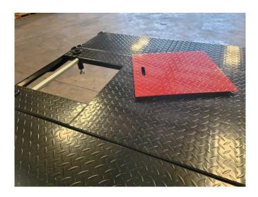
To operate the casters and roll the lift around your shop, use a large allen key to turn clockwise on the caster post shown below. Spin the caster downward at each corner until all four casters are supporting the weight of the table and the frame of the table is no longer touching the ground. "DO NOT" attempt to lower the casters if the lift table is loaded as this will surely destroy the casters. The casters are only strong enough to support the table itself, and nothing more.
