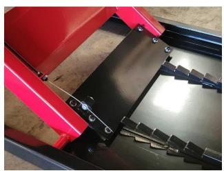
The drop out panel is easily installed and removed with no tools or hardware. Notice in this picture below that the side extension support pole runs through the drop out panel, effectively rendering the drop out panel ineffective for rear wheel removal. For this reason, rear tire changes are typically not possible if the side extensions are installed, so be sure to leave them off the table if this is your intent.
