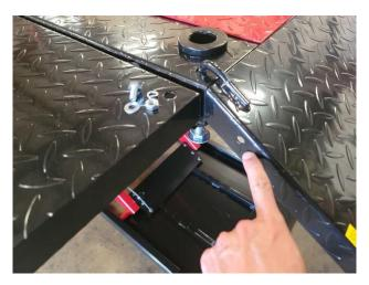
If you purchased the optional wheel vise with your trike lift, both your table and your front extension panel come pre-drilled with the necessary mounting holes to install the Redline wheel vise to this table as shown. Be sure to use ratchet straps to secure your bike to the lift as the wheel vise alone is not sufficient to hold the motorcycle firmly to the lift.
