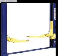
Asymmetrical arm design attached to two symmetrical columns, making for one very rugged lift.
