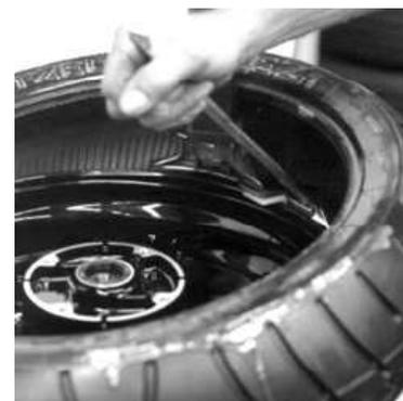
heavily corroded wheels. Inspect tire for damage, paying close attention to the beads. Verify size match between tire and wheel.
